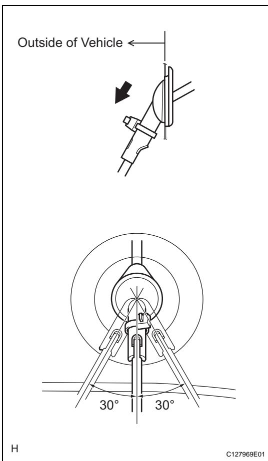
(f) Hold the grommet and pull it from the inside of the vehicle to the outside of the vehicle. Then fix it in place so that it is not tilted.
