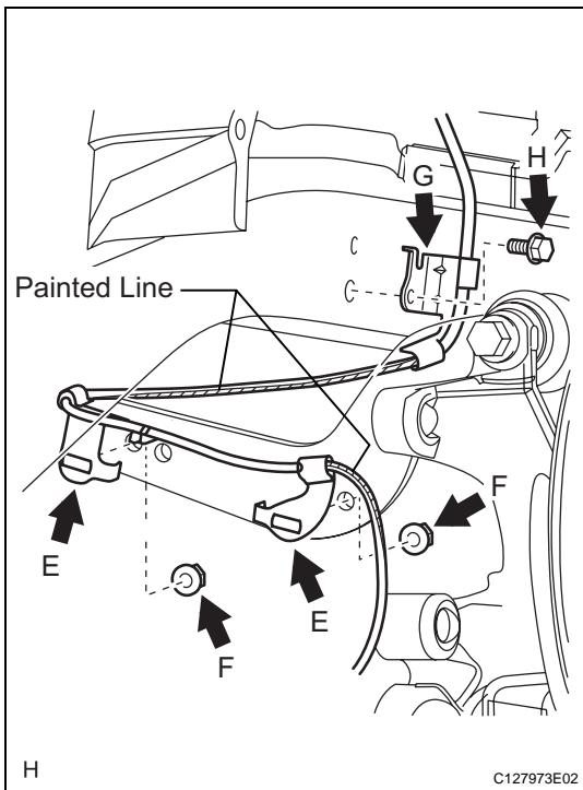
(c) Install the sensor clamps (labeled E) with the 2 nuts (labeled F).
