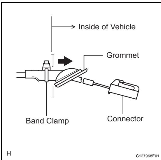
(e) Insert the connector and grommet to the inside of the vehicle through the passage hole in the wheel house.
